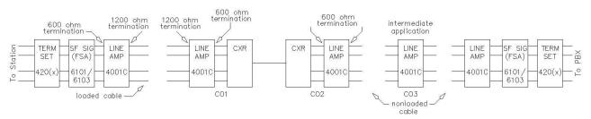
FIGURE 5. Typical 4Wire DX Signaling Application Using 104001C Line Amplifiers.
